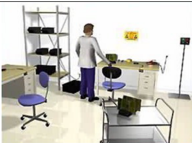
example of an electrostatic protected area (epa) set up source: www.armeka.com
