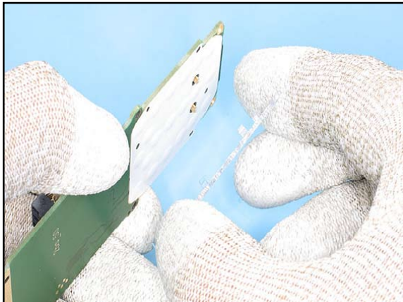
16. If both sides are clearly unlocked, the KEYMAT LIGHT GUIDE ASSY can be removed easily.
