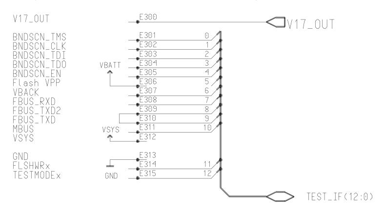
VBATT should connect together with XIP Flash VPP Which is separately routed from frame connector
