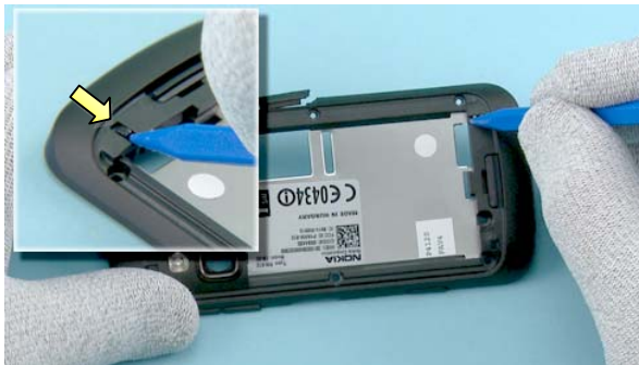
35) To remove the ANTENNA ASSEMBLY, push the shown clip with the sharp end of the SS-93.
