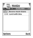
Fill in the fields. Use (•) to move between fields. Alarm (meetings and anniversaries)—Select On, and press to fill in the Alarm time and Alarm date fields. ? in the day view indicates an alarm.
