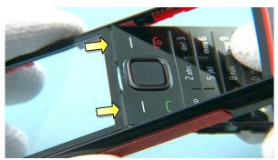
9) Make sure that the KEYPAD covers the bottom end of the A-COVER window shown by the arrows.
