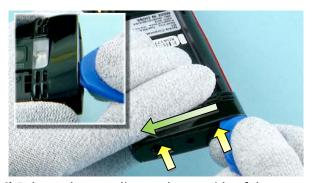
6) Release the two clips on the top side of the device by sliding the SRT-6 to the direction shown.
