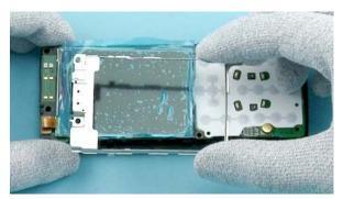
27) Lift up the UI SHIELD and remove it.
