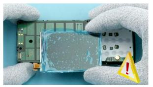
30) Remove the LCD DISPLAY carefully.
