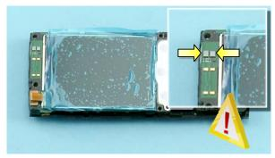
28) Be careful not to damage the two ASIP components during disassembly.
