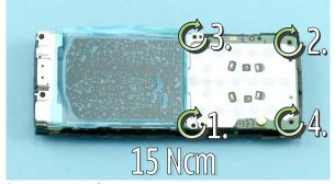
7) Tighten the four TORX + size 6 screws to the torque of 15 Ncm in the order shown.
