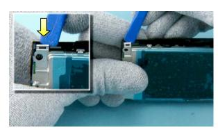
23) Release the first clip of the UI SHIELD with the SS-93.
