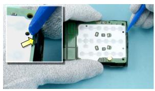
30) Release the clip holding the LIGHT SWAP PWB using the SS-93.
