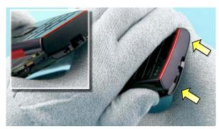
16) Open the remaining two clips on the bottom side of the phone.
