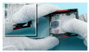
19) Press out the KEYPAD from the A-COVER ASSY as shown.
