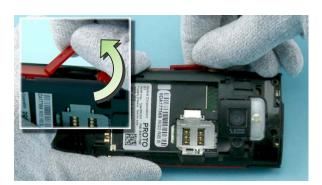
11) To remove the A-COVER ASSY, first open the SD card door.
